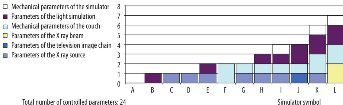
Figure 9. Number of parameters beyond accepted tolerance limits for particular simulators tested.
