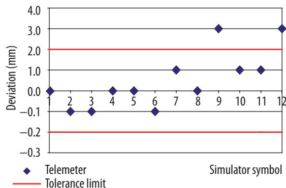
**Figure 3.** Deviation of the telemeter indications from the nominal value of SSD=100cm.
