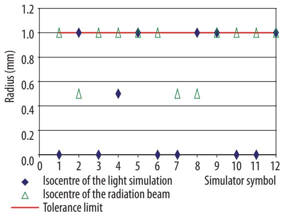
**Figure 1.** The size of the isocentre of the radiation and light beams.
