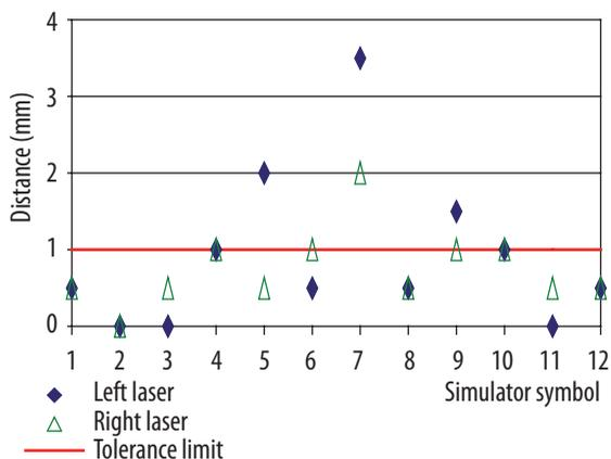
**Figure 2.** Distance between vertical line of the side laser and the isocentre of the light beam.
