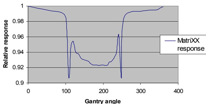
**Fig. 7.** Response of MatriXX with angle of irradiation
