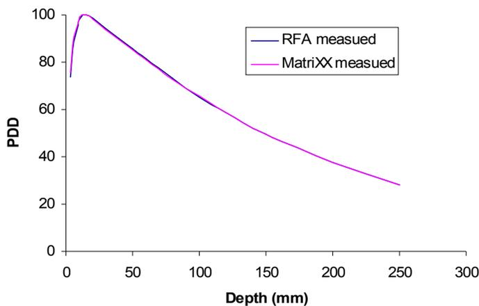
**Fig. 3.** PDD measurement comparison between RFA-300 and MatriXX
