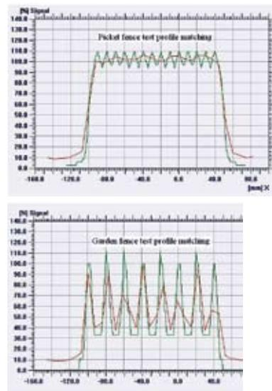
**Fig. 5.** Profile matching between TPS and MatriXX measurement along X direction for Picket and Garden fence test.
